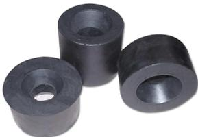
Foundation Buffers are rubber moulded products which are usually manufactured in special rubber compounds to provide resistance to overheating of the rubber in the dynamic application. Used on screens and conveyors they provide excellent vibration isolation to the surrounding structure. Stiffness is controlled by rubber hardness and dimensions with the possibility to alter the internal profile. Many sizes and configurations are available from a diameter of 95mm up to 250mm.
