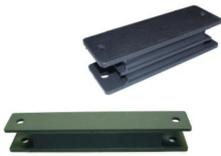
Sandwich Mounts consist of rubber bonded between two plates and are often mounted in shear or at an angle to take advantage of the appropriate stiffness properties in the direction of movement. Stiffness properties can be controlled by both rubber hardness and inserting metal interleaves. Many different sizes and configurations are available and parts can be specified to meet the application requirements where needed.
