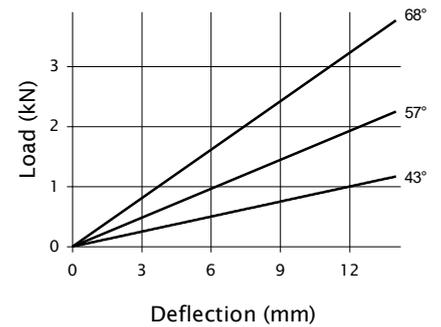
Note: There is a possible deviation of ±20% in the above load/deflection graphs due to production and hardness tolerances
