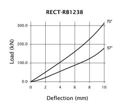
$Note: There \ is \ a \ possible \ deviation \ of \ \pm 20\% \ in \ the \ above \ load/deflection \ graphs \ due \ to \ production \ and \ hardness \ tolerances$
