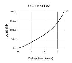
$Note: There \ is \ a \ possible \ deviation \ of \ \pm 20\% \ in \ the \ above \ load/deflection \ graphs \ due \ to \ production \ and \ hardness \ tolerances$
